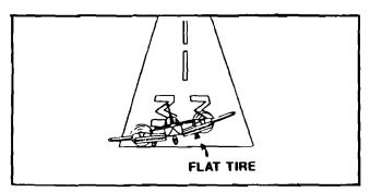
If a nosewheel is flat or the nose gear won't extend, you may want to carefully shift weight aft (within limits, of course) to help hold the nose off the runway until the aircraft slows. Passengers can move to rear seats if these seats are empty!
