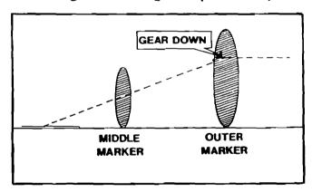
For localizer and VOR approaches, the gear should be extended when passing the final approach fix (FAF) inbound.
