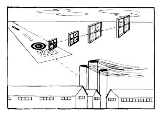
Your last and most important window is the one at the runway threshold. You should be at the required airspeed and height to complete the landing when you pass through this last window.
