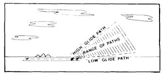
Select a glide path that works best for a particular situation, but make sure it allows for clearance of all obstacles and for a *safe* rate-of-descent.
