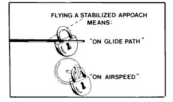
Make your normal pattern entry and extend your landing gear on downwind, if applicable. Abeam the intended landing point, reduce your power to the predetermined value that works best for your airplane. While holding altitude with pitch, slow the airplane down in preparation for turning base.
