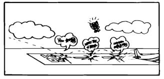
Ground effect, a factor from the surface to a height of about half the plane's wing span, decreases elevator control effectiveness and increases the effort required to raise the nose and hold the airplane off. Not enough elevator (or stabilator) trim can result in a nose-low contact with the runway and a porpoise.
