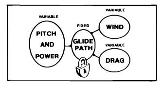
Then, these pilots need only make minor adjustments to pitch and power to maintain the selected glide path and airspeed.
