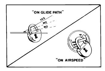
You should now be able to hold the selected airspeed and set up a stabilized rate-of-descent. With the runway in sight, and a landing assured, extend final landing flaps. Retrim again and maintain positive control of the aircraft, since adding flaps without promptly retrimming could possibly cause you to "balloon" back into the clouds.
