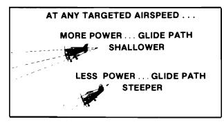
This inter - relationship means that any changes to one element in the "approach equation" must be compensated for by adjustments in the other.
