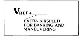
"Approach segment airspeeds," based on V-ref, assure that the aircraft has just the right amount of extra airspeed margin above V-ref.
