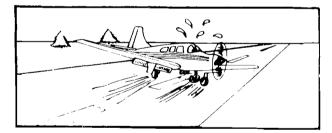
Proper crosswind technique is a must. In the case of a left crosswind, the left wing must be lowered into the wind and this control input countered with right rudder to maintain the proper track down to the runway. Again, the longitudinal axis of the airplane must be aligned with the flight path which, hopefully, is parallel to the runway centerline.
