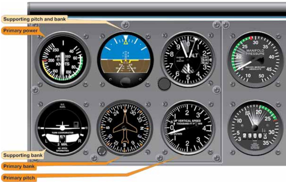
Figure 5-30. Constant Airspeed Descent, Airspeed High—Reduce Power.
