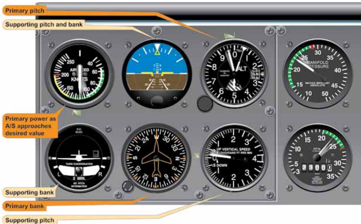
Figure 5-29. Level Off at Cruising Speed.
