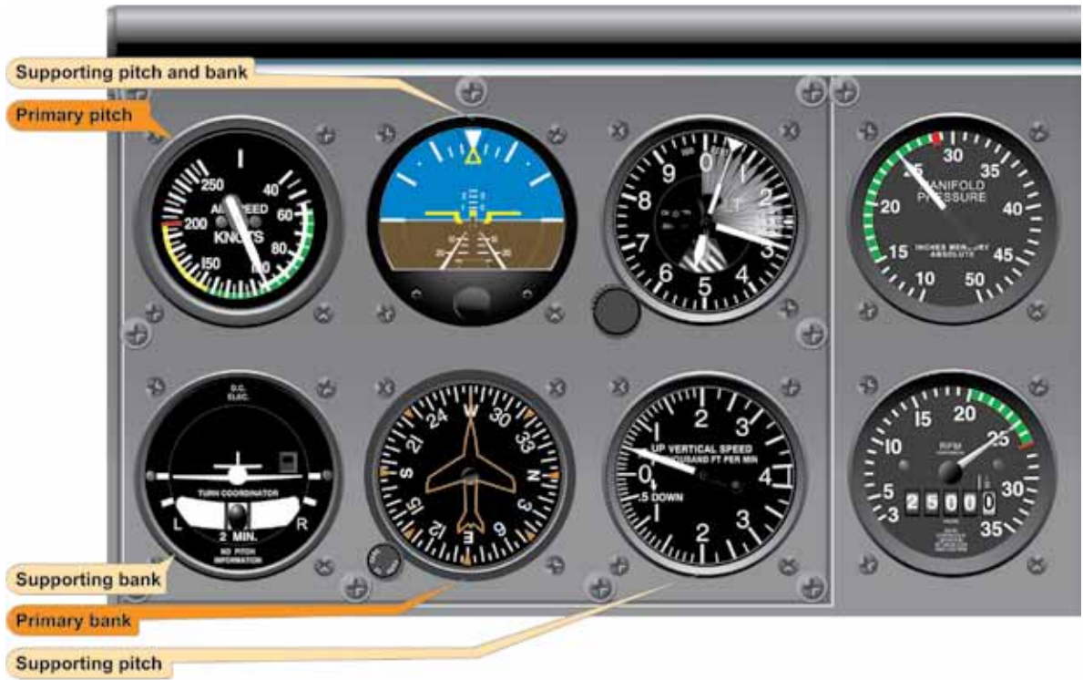
Figure 5-26. Stabilized Climb at Constant Airspeed.
