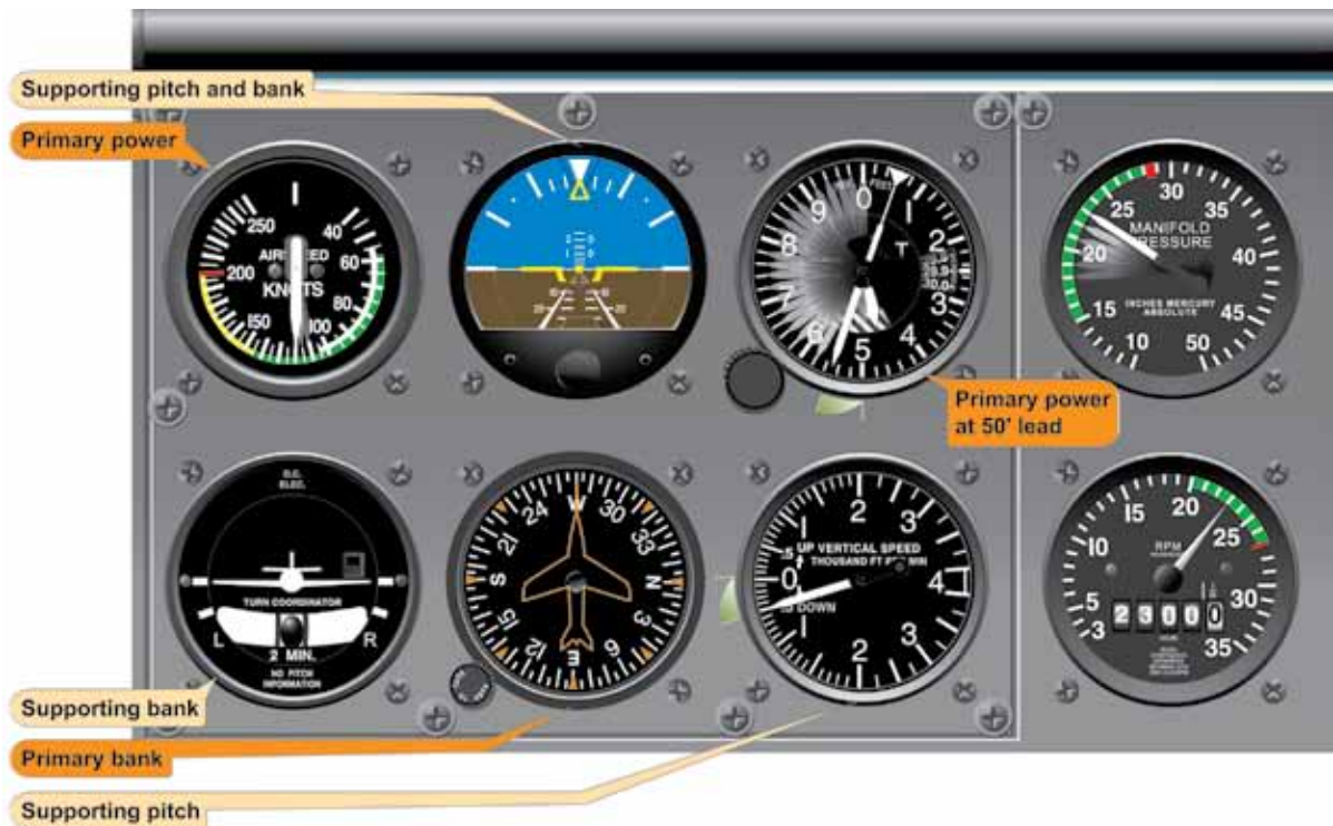
Figure 5-32. Level Off at Descent Airspeed.
