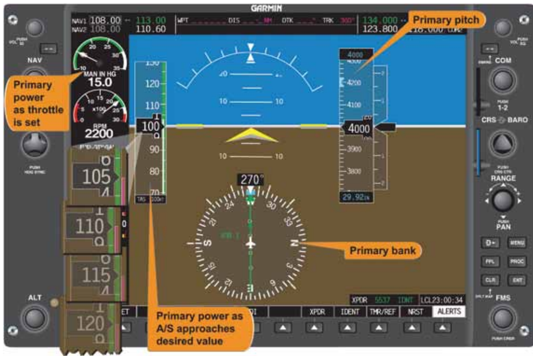
Figure 5-58. Straight-and-Level Flight (Airspeed Decreasing).
