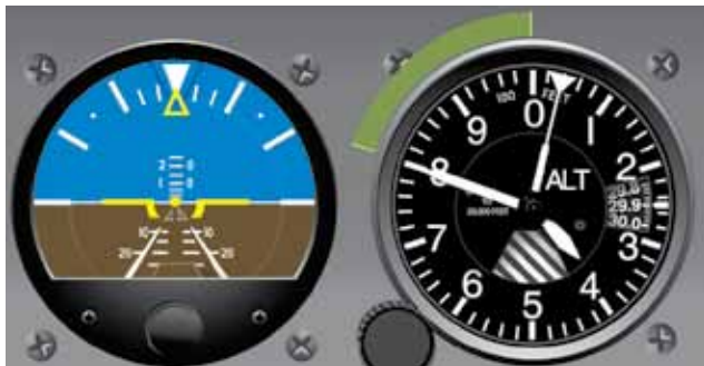
Figure 5-11. Altitude Error, Greater Than 100 Feet.
