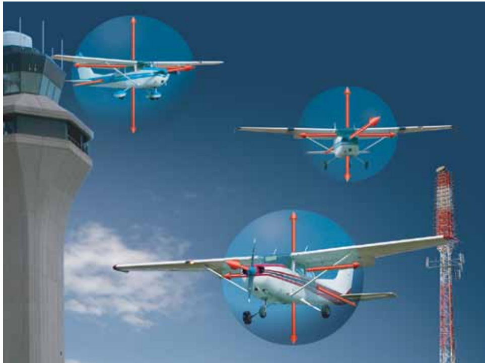
Figure 3-48. Aircraft equipped with Automatic Dependent Surveillance—Broadcast (ADS-B) continuously broadcast their identification, altitude, direction, and vertical trend. The transmitted signal carries significant information for other aircraft and ground stations alike. Other ADS-equipped aircraft receive this information and process it in a variety of ways. It is possible that in a saturated environment (assuming all aircraft are ADS equipped), the systems can project tracks for their respective aircraft and retransmit to other aircraft their projected tracks, thereby enhancing collision avoidance. At one time, there was an Automatic Dependent Surveillance—Addressed (ADS-A) and that is explained in the Pilot's Handbook of Aeronautical Knowledge.
