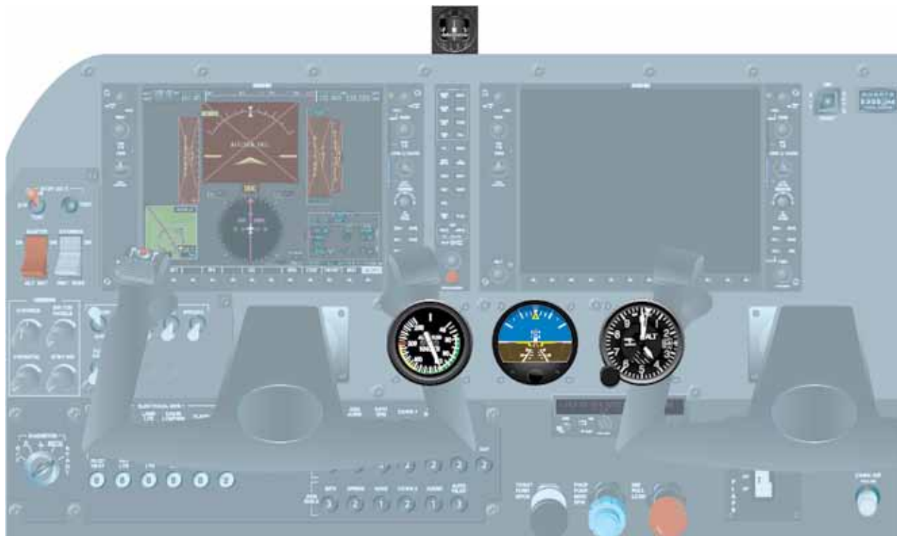
Figure 11-7. Emergency Instrumentation Available to the Pilot on Electronic Flight Instrumented Aircraft.
