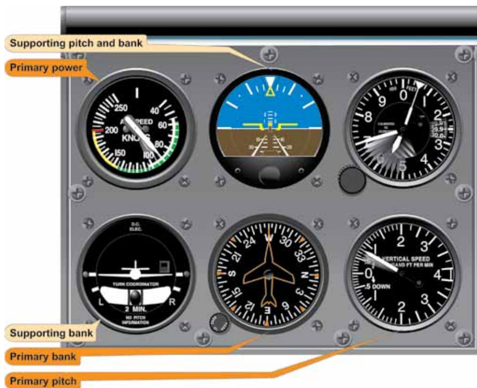
Figure 5-28. Airspeed Low and Vertical Speed High—Reduce Pitch.
