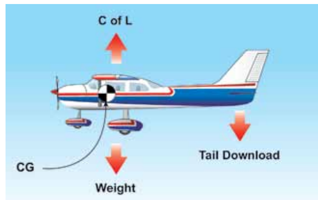
Figure 2-21. Downward Force on the Tailplane.
