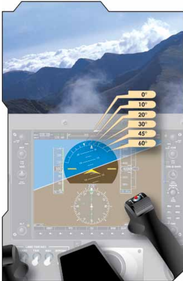
Figure 4-29. Bank Control Index Lines.
