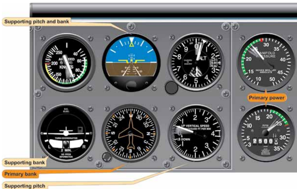
Figure 5-25. Climb Entry for Constant Airspeed Climb.
