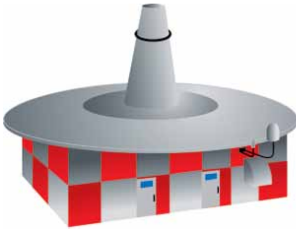
Figure 7-11. VOR Transmitter (Ground Station).
