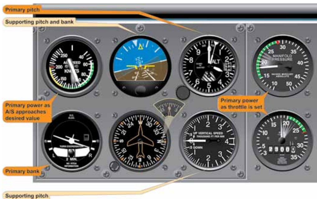
Figure 5-38. Change of Airspeed During Turn.
