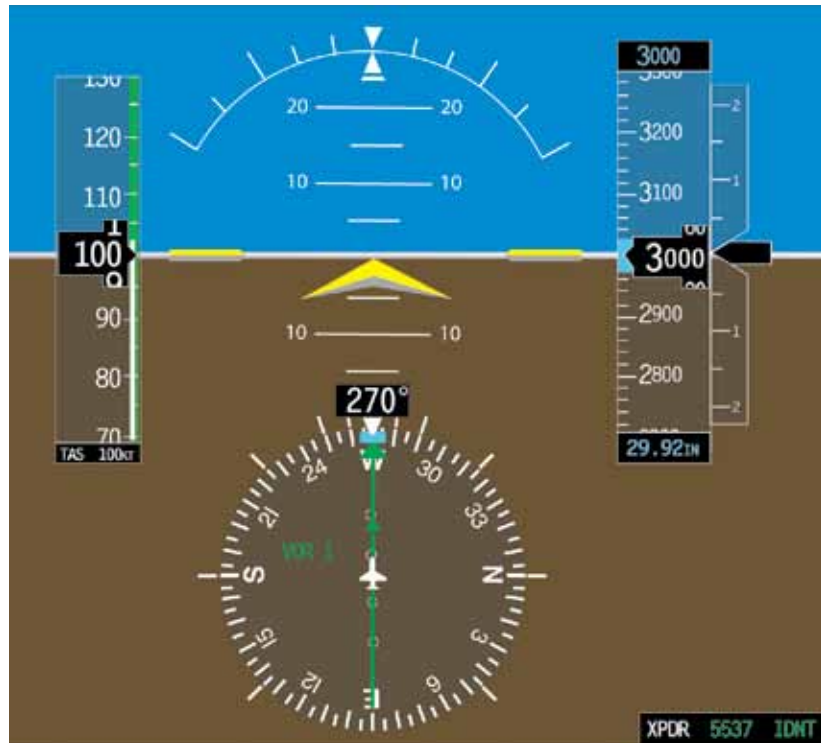
Figure 6-17. PFD Indications During Straight-and-Level Flight.
