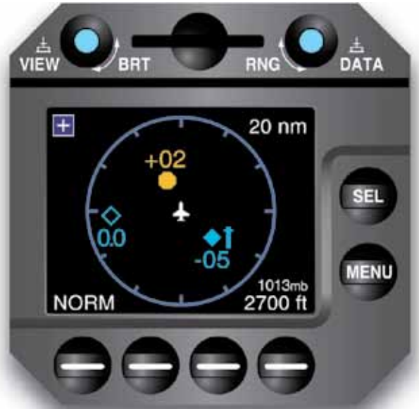
Figure 3-56. A Skywatch System.
