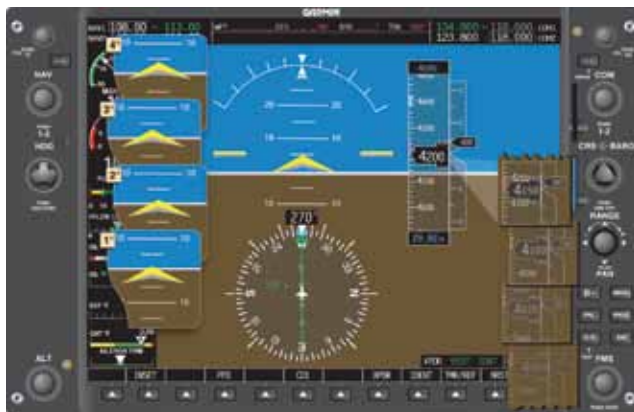
Figure 5-50. Pitch Indications for Various Attitudes (1° through 5°).
