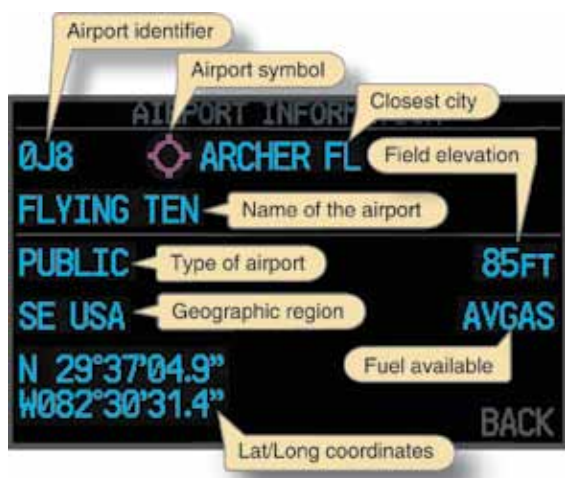
Figure 11-12. Information shown on the additional information page that will aid the pilot in making a more informed decision about which airport to choose when diverting.
