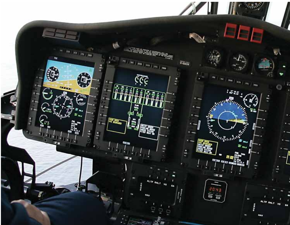
Figure 6-20. MFD Display of Aircraft Systems.
