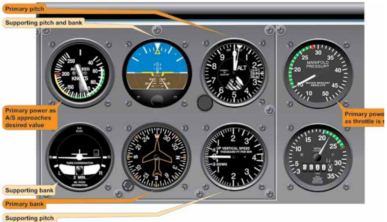
Figure 5-23. Straight-and-Level Flight (Airspeed Decreasing).
