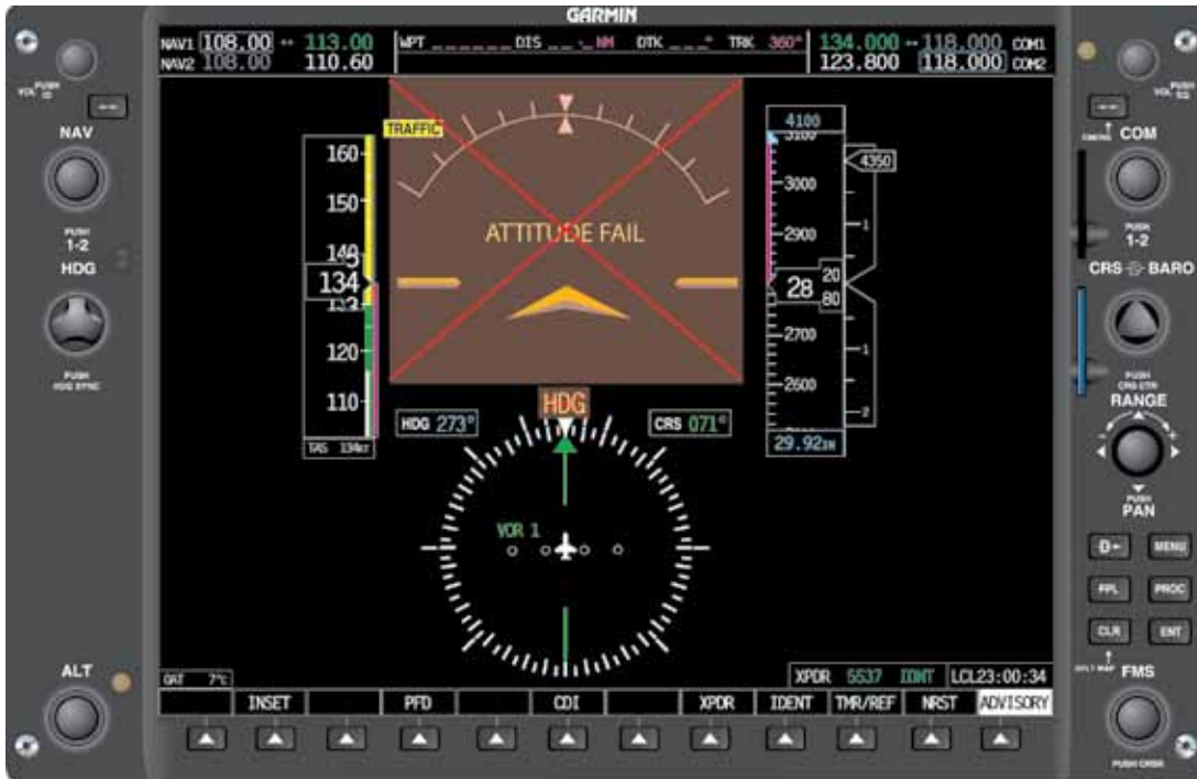
Figure 5-73. AHRS Unit Failed.
