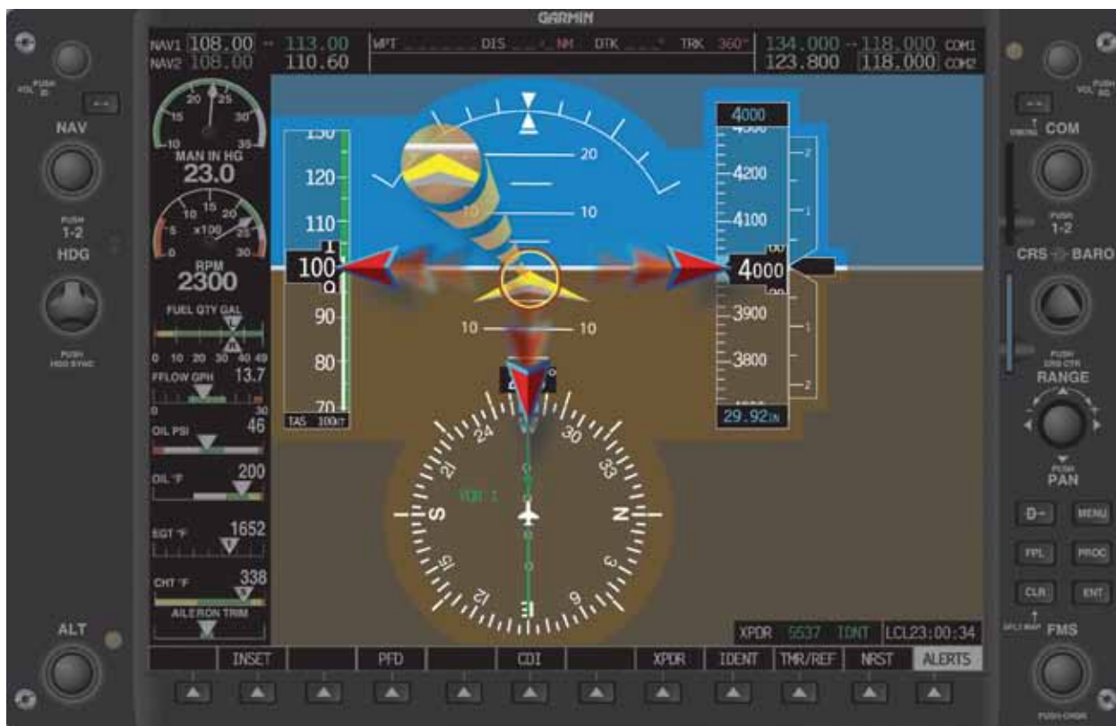
Figure 5-60. Cross-check Supporting Instruments.
