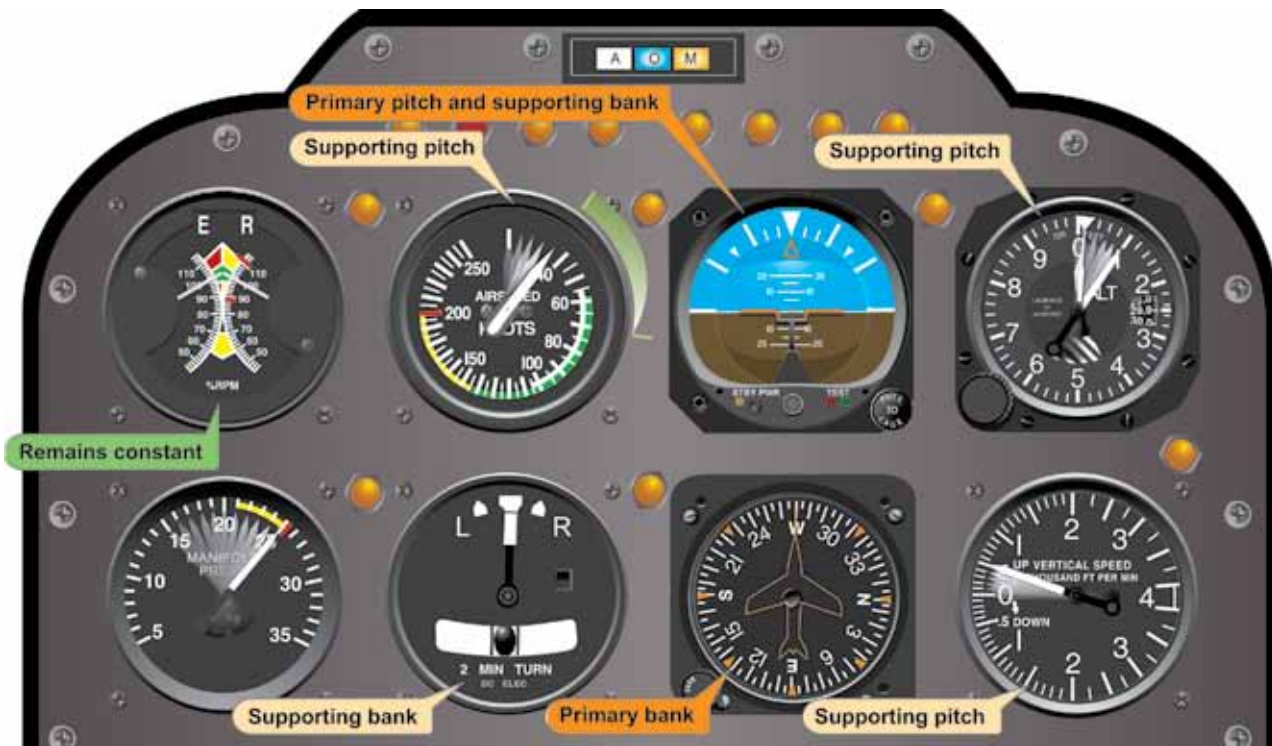
Figure 6-16. Flight Instrument Indications During an Instrument Takeoff.
