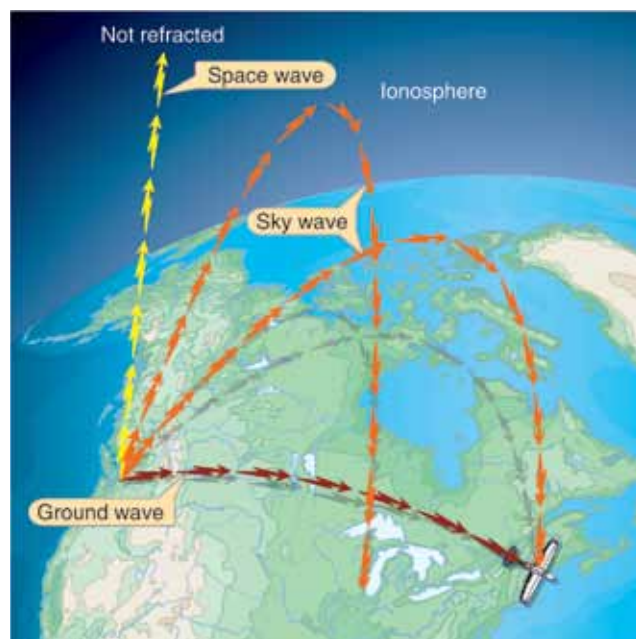
Figure 7-1. Ground, Space, and Sky Wave Propagation.
