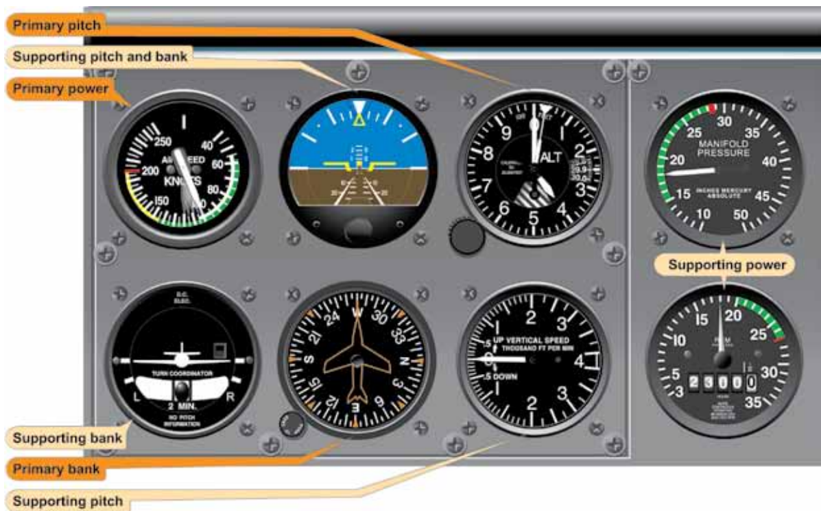
Figure 5-24. Straight-and-Level Flight (Reduced Airspeed Stabilized).
