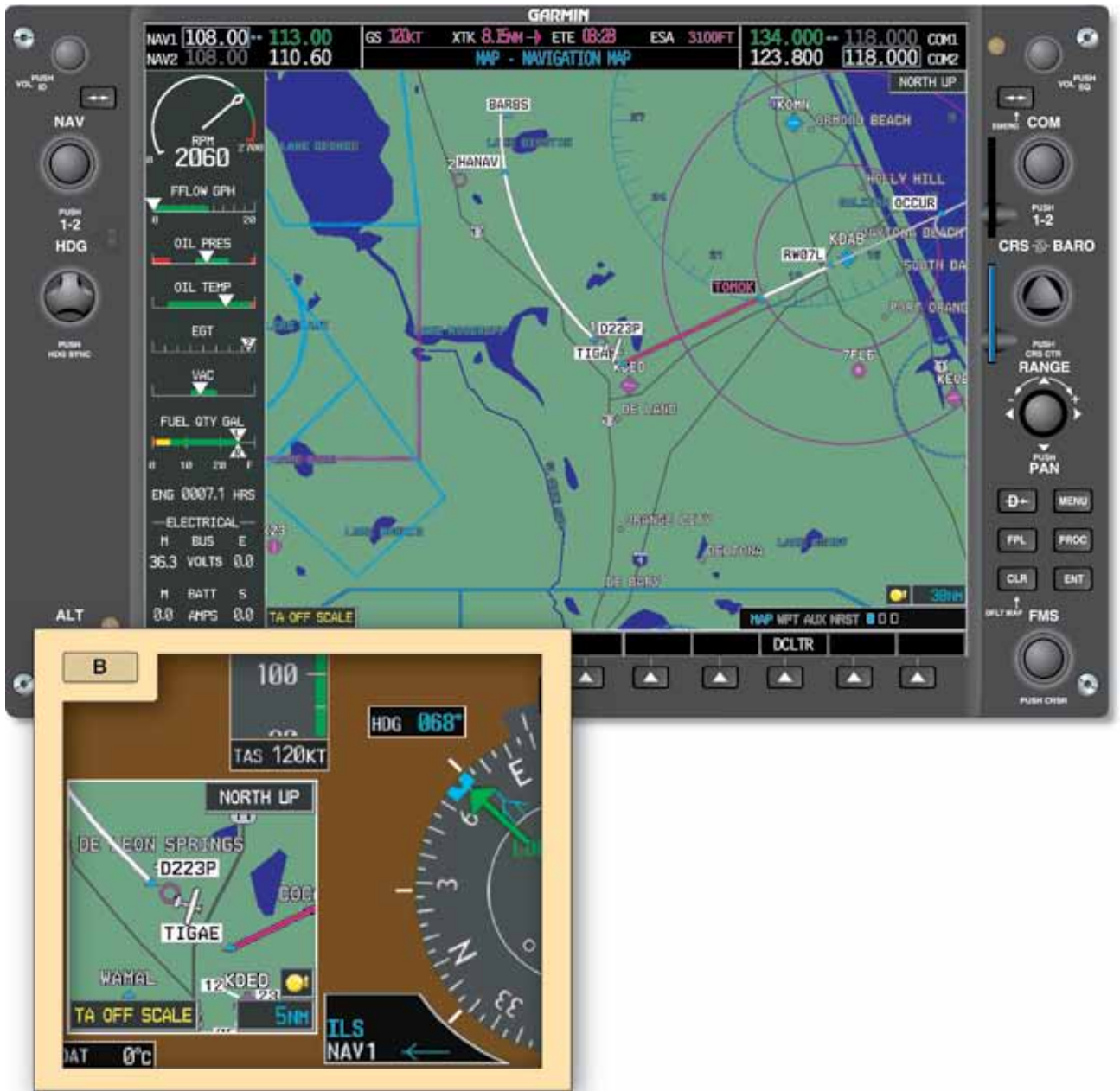
Figure 7-20. The same aircraft illustrated in Figure 7-19 shown on the ORM radial near TIGAE intersection turning inbound for the localizer.
