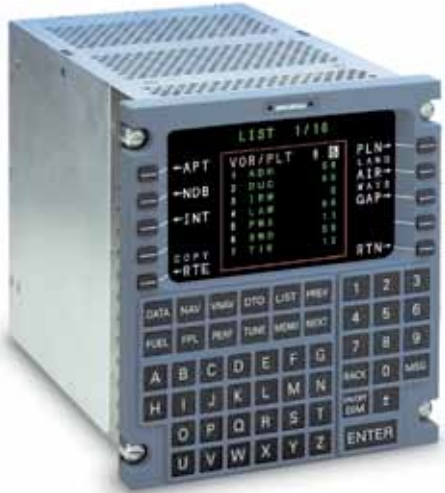
Figure 3-44. A Control Display Unit (CDU) Used to Control the Flight Management System.
