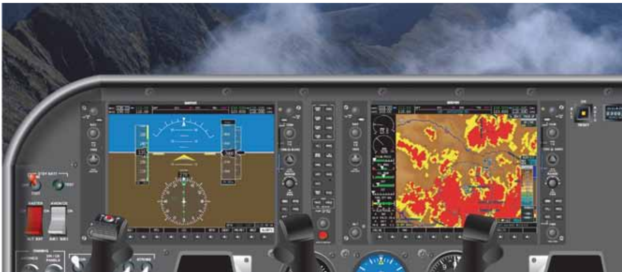
Figure 5-48. Pitch Attitude Decreasing and Airspeed Increasing—Indicates Need to Increase Pitch.
