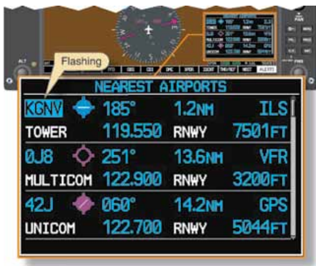
Figure 11-10. An enlargement of the box shown in the lower right of Figure 11-9. Note that KGNV would be flashing.
