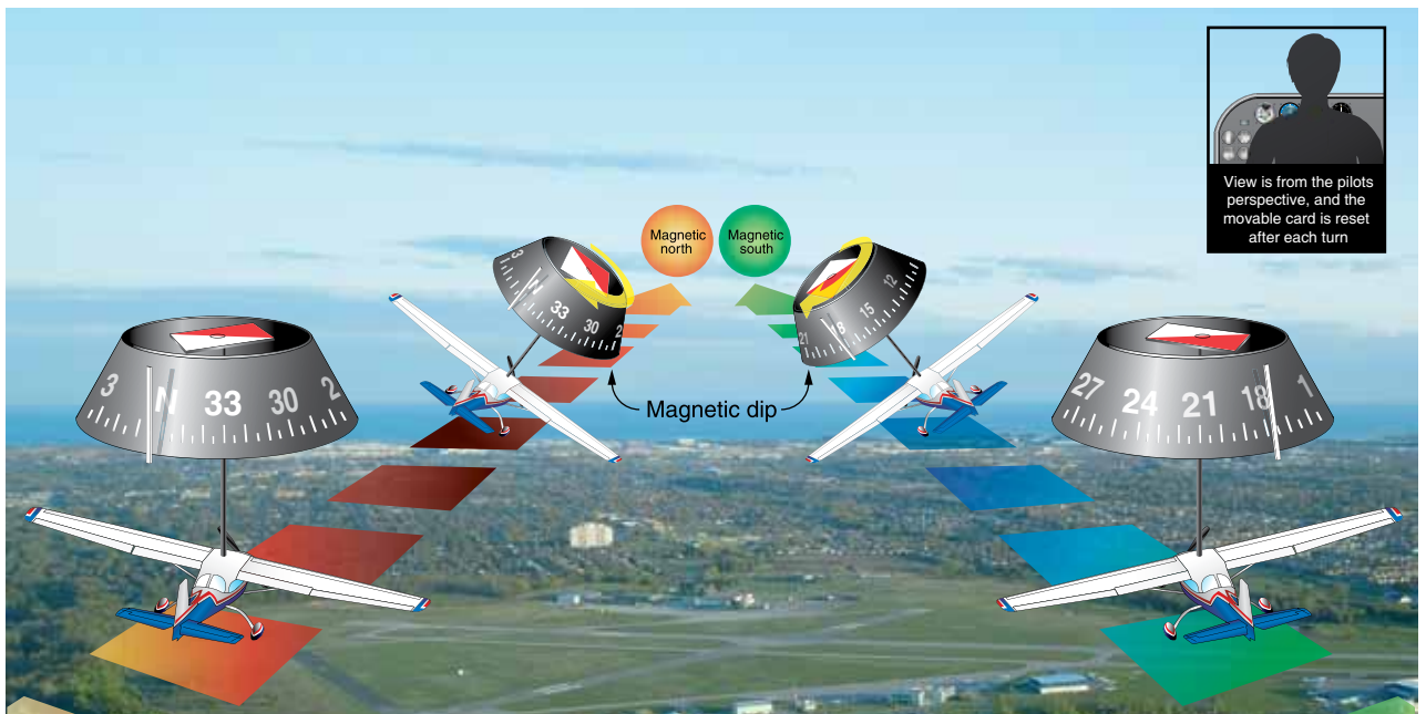
Figure 3-20. Northerly Turning Error.
