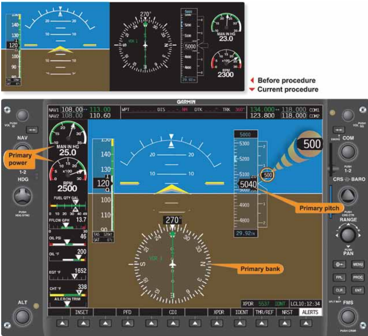
Figure 5-63. Constant Airspeed Climb From Cruise Airspeed.
