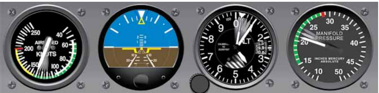
Figure 5-21. Airspeed and Altitude High—Lower Pitch and Reduce Power.
