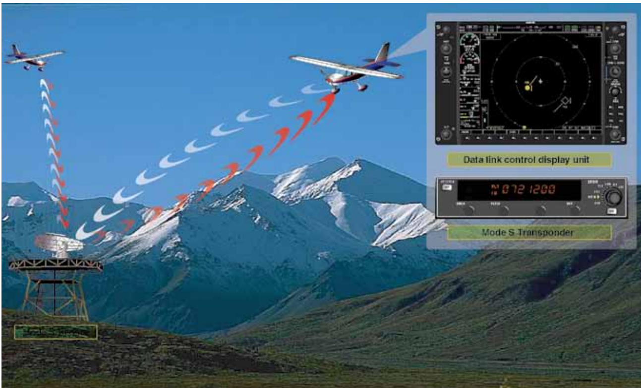
Figure 3-54. Concept of the Traffic Information System.
