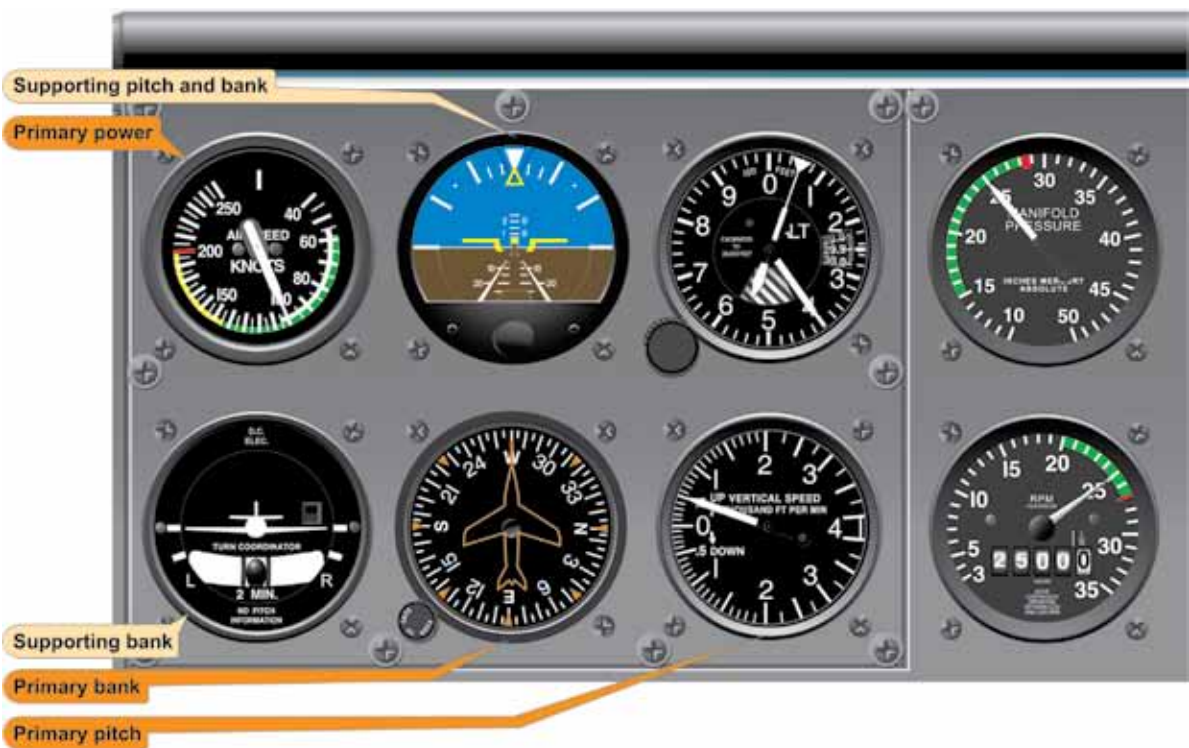
Figure 5-27. Stabilized Climb at Constant Rate.
