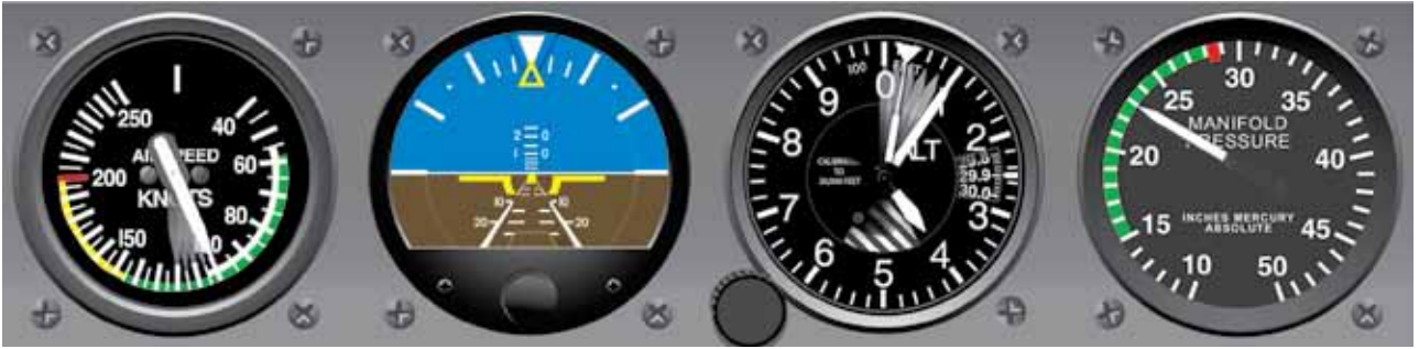
Figure 5-20. Airspeed Low and Altitude High—Lower Pitch.
