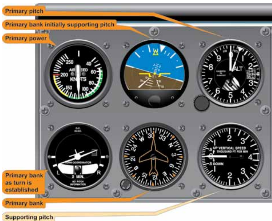
Figure 5-33. Standard Rate Turn, Constant Airspeed.
