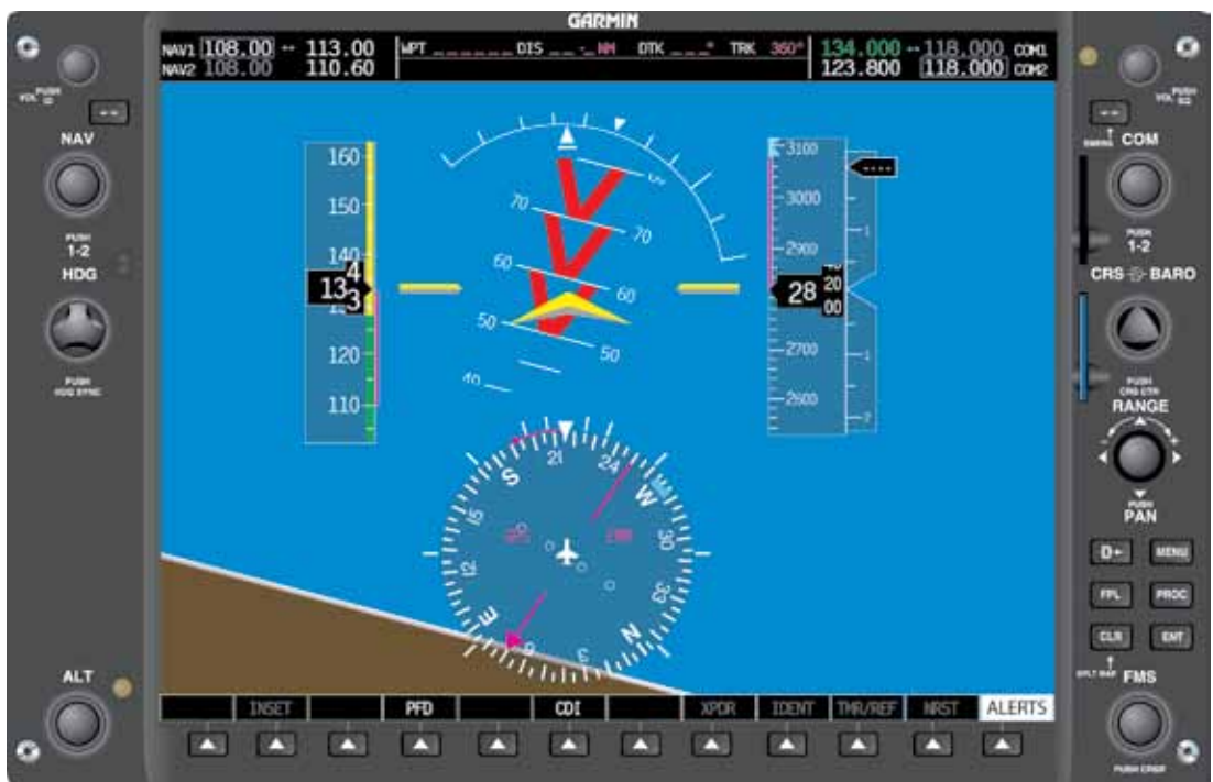
Figure 5-72. Unusual Attitude Protection With Valid AHRS.
