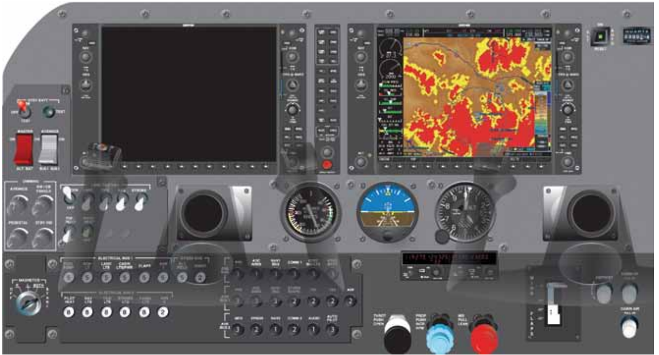
Figure 4-22. Multifunction Display (MFD).
