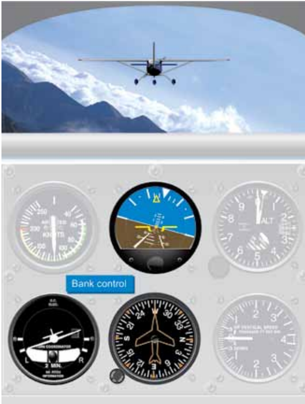
Figure 5-16. Instruments Used for Bank Control.
