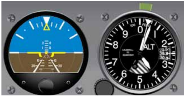
Figure 5-9. Altitude Error, Less Than 100 Feet.
